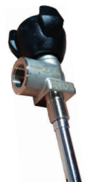
Sanosub Italy Flow rate : 950 to 1400L/M M 8x0.75, 10Nm Torque Suitable for 200 and 300 bar
